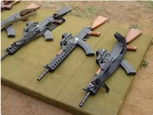
The handguard has a very long travel Picatinny rail
